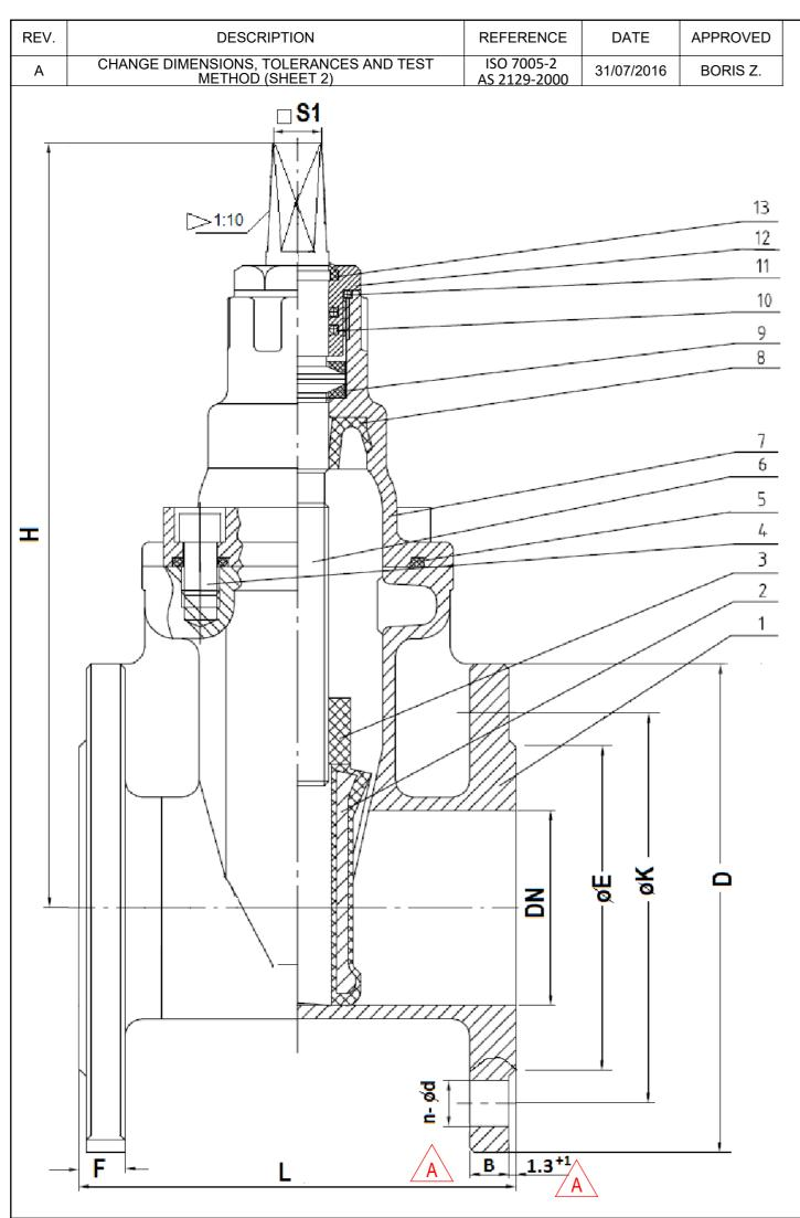
Dwg: G:\DEVELOPMENT\GATE VALVES [RED STAR-KGV]\2"-12" GATE VALVES\_RevA; Model: \*Model Rev:
