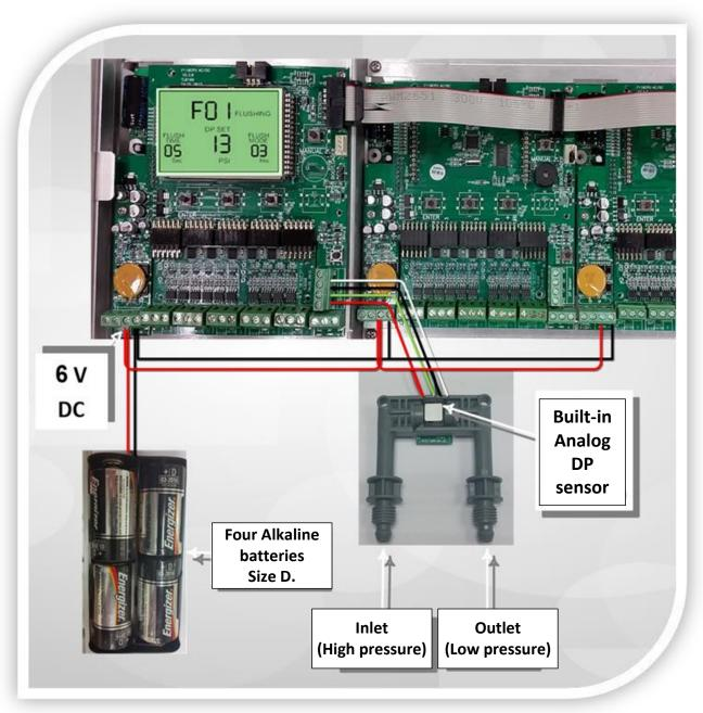
Filtron 20 30 DC: Outputs and inputs wiring.
