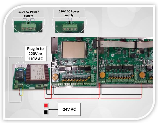
Filtron 20 30 AC: Energy wiring.
